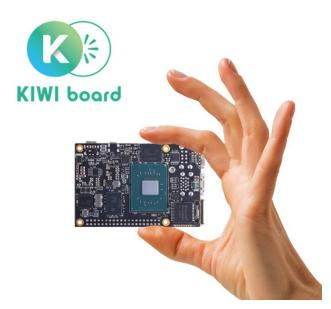
Accordingly, Axiomtek presents the smallest x86 embedded SBC, KIWI310. Its size is as small as a kiwi or a credit card, and it's being recognized as an excellent choice for space-constrained environments.
