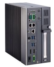
M.2 Key B+M 2280 socket. Also, it has two DDR4-3200 unbuffered SO-DIMM slots that can support up to 64GB of system memory. The front I/O includes four USB 3.1 type A ports, one 2.5G LAN and two GbE LAN ports, one RS-232/422/485 COM port, and a programmable 8 CH DIO. Users can expand the I/O via the flexible window with COM or LAN modules.
